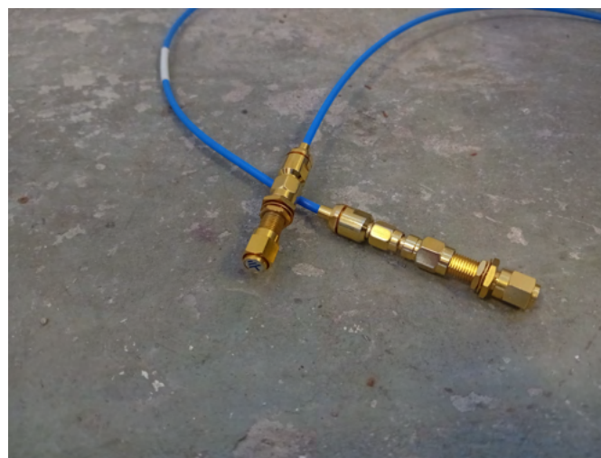
Figure 11: Shorted ends on the wires connecting to the antenna.
