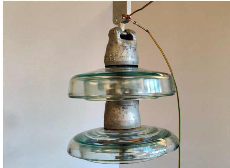
Figure 7: Insulator chain with two bells.
