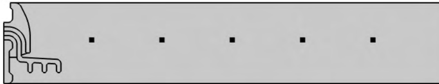
Figure 3: Geometry of insulator bell that was investigated, the free floating squares seen beside the insulator bell is measurement points where the electric field levels will be recorded.
